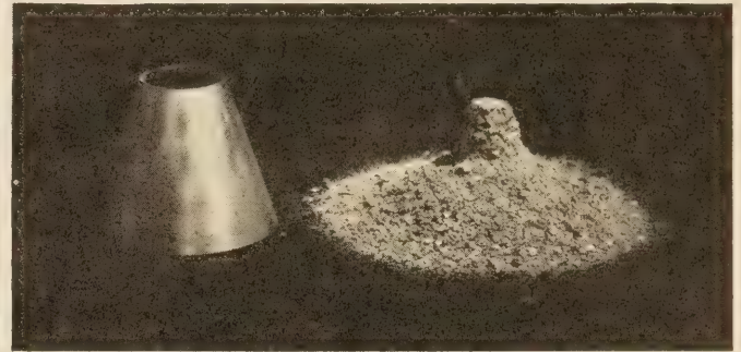
FIGURE 1.—STEPS IN PERFORMING THE CONE TEST ON SAND. LEFT; TAMPING MOIST SAND IN THE CONE. UPPER RIGHT; THIS SAND CONE RETAINED ITS SHAPE INDICATING THE PRESENCE OF FREE MOISTURE. LOWER RIGHT; THIS SAND CONE SLUMPED, INDICATING THAT THE MATERIAL HAD REACHED A SURFACE-DRY CONDITION.
